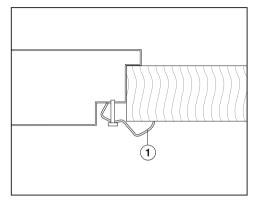
■ Secure the cooktop at the **front** and **rear** with fixing brackets, ①, (supplied) as shown.
